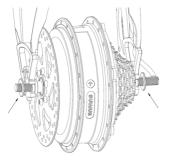
6. Fasten two M12 flange nuts with open-end wrench at both ends of the motor. Torque requirement: 47-60N.m.
